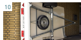
10 STORAGE BRACKET ON WHEELS | Store your camper upright to save space.
