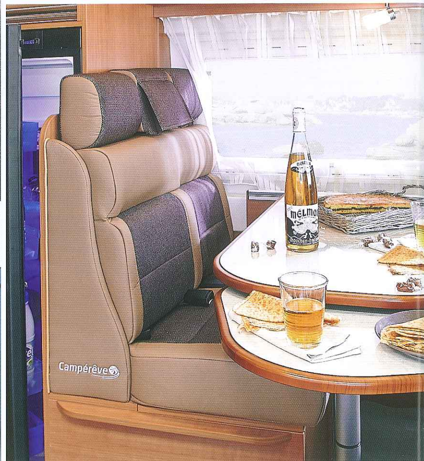
SELLERIE CAMPÉRÈVE MOUSSÉE ET TISSU DOUBLE PIQURE CAMPÉRÈVE UPHOLSTERY WORK, FOAM AND FABRIC DOUBLE STITCHED
