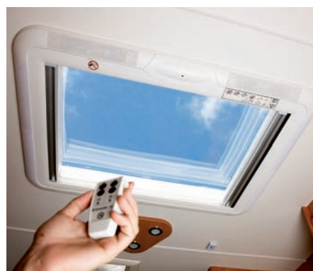
Automatic rain-sensitive Heki rooflight
